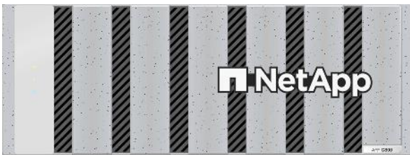
Figure 27. NetApp AFF C800 Front View
