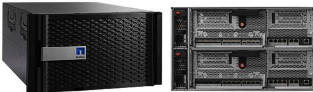
Figure 8 NetApp FAS8040/8060 (6U) - Front and Rear View
