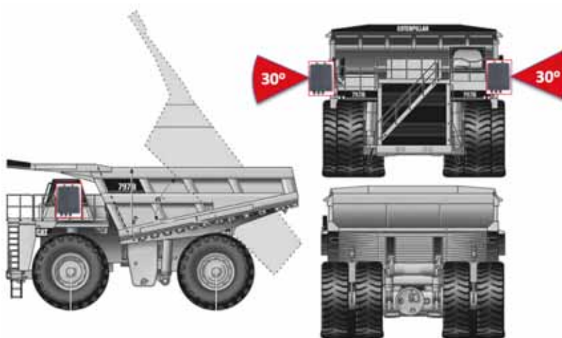
Figure 47 Hauler onboard setup - Dual Radios with directional antennas
