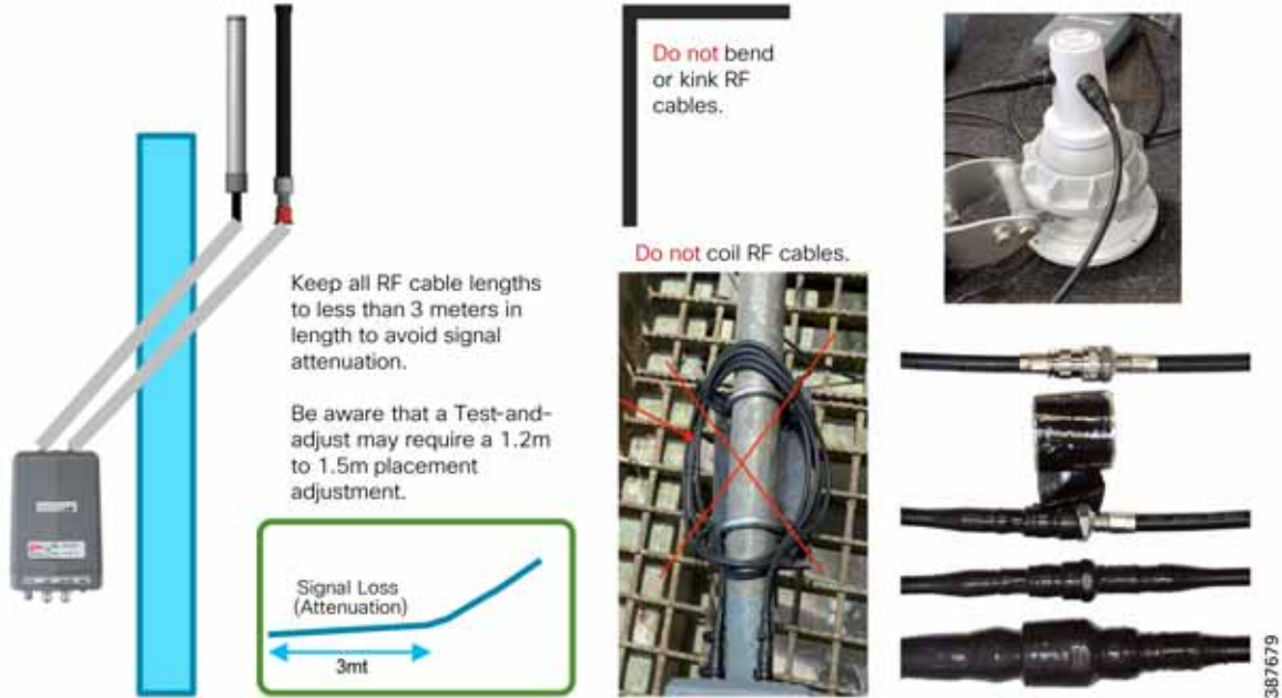
Figure 56 Cabling Installation Best Practices
