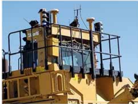
Figure 52 Example of Dozer with a Single Radio and OMNI-5-KIT Antenna installed on the top
