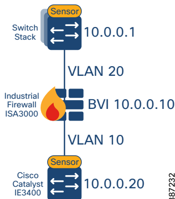
Figure 21 Transparent Mode with BVI Interface
