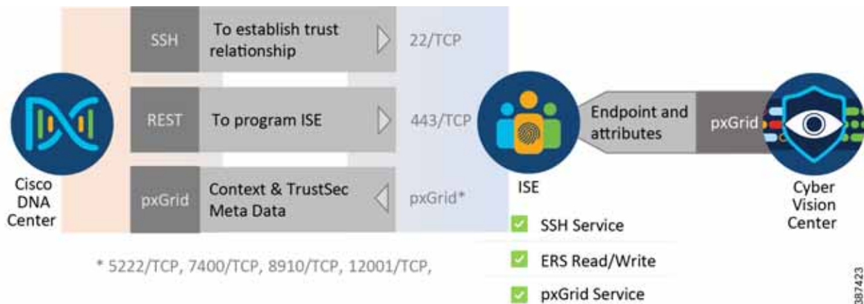
Figure 4 Cisco DNA Center, ISE, and Cisco Cyber Vision Integration
