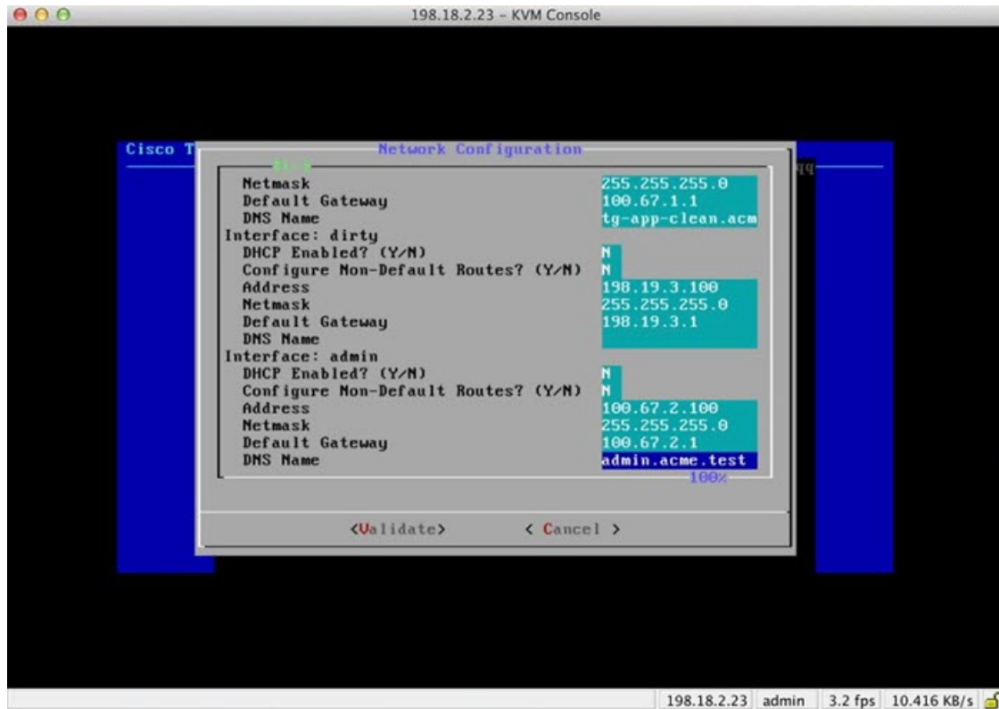
Figure 11: Network Configuration In-Progress (Admin)
