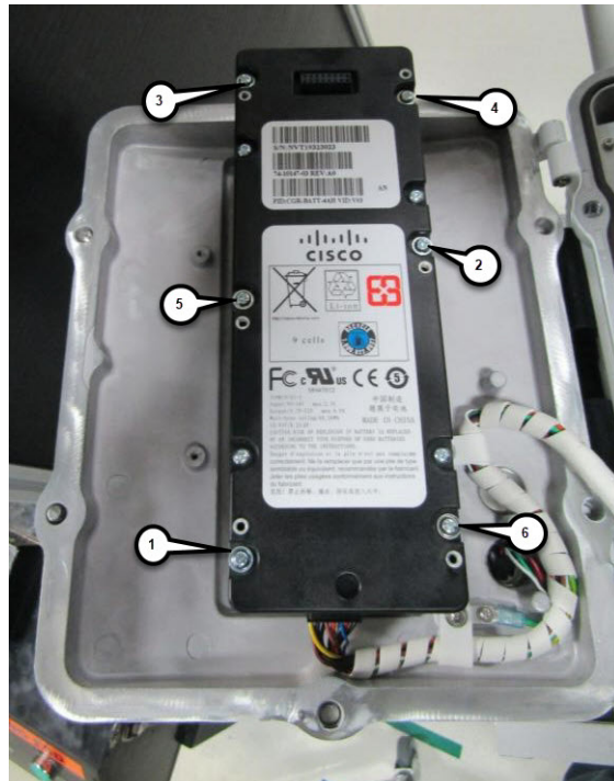
Figure 12 Sequence of Tightening and Loosening BBU Screws
