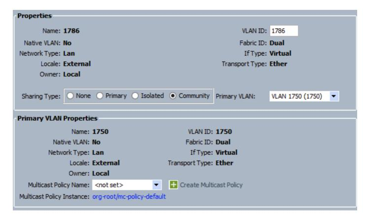
3. Virtual Network Interface Card (vNIC) on service-profile carries regular VLANs as well as PVLANs, as seen in the image.
