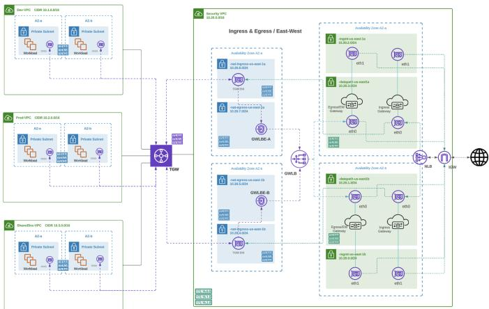
**Figure 2.**Centralized Ingress Deployment Architecture (AWS)
