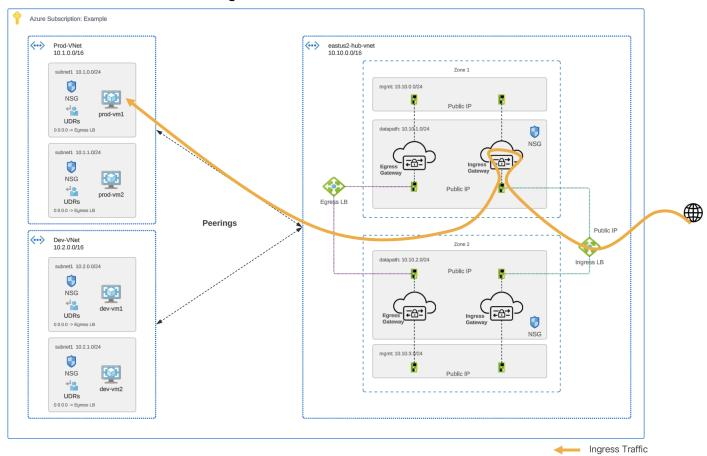
**Figure 13.**Azure Centralized Ingress - Traffic Flow
