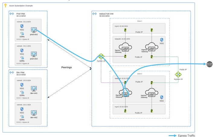
**Figure 15.**Azure Centralized Egress - Traffic Flow
