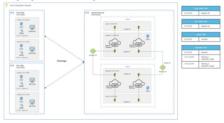
**Figure 14**. Azure Centralized Ingress - Routing Configuration
