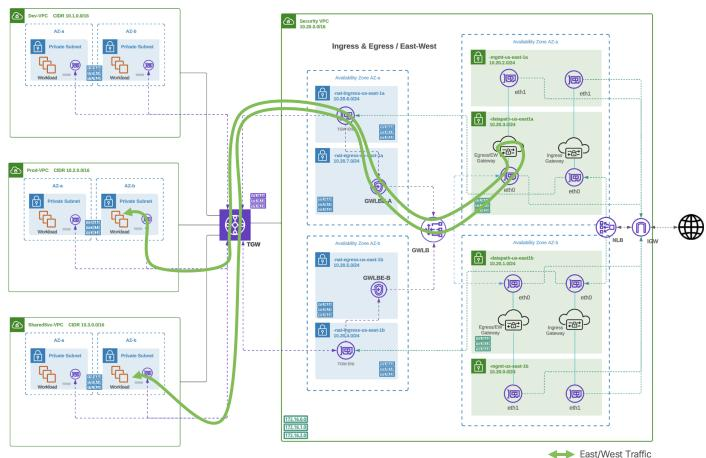
**Figure 6.**Traffic Flow Centralized East-West, Inter-VPC (AWS)
