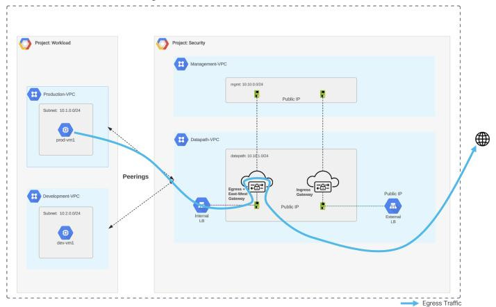
**Figure 20.** GCP Centralized Egress – Traffic Flow
