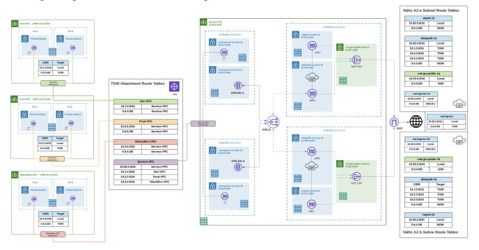
**Figure 11.**AWS Centralized Egress / East-West (NAT Gateway) - Routing Configuration
