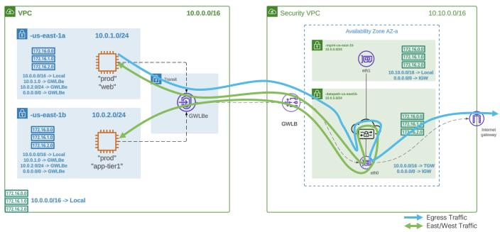
**Figure 7.**Traffic Flow Centralized East-West, Intra-VPC (AWS)
