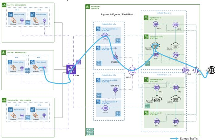
**Figure 5**. Centralized Egress Traffic Flow - Egress (AWS)
