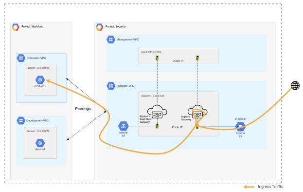
**Figure 18.** GCP Centralized Ingress – Traffic Flow
