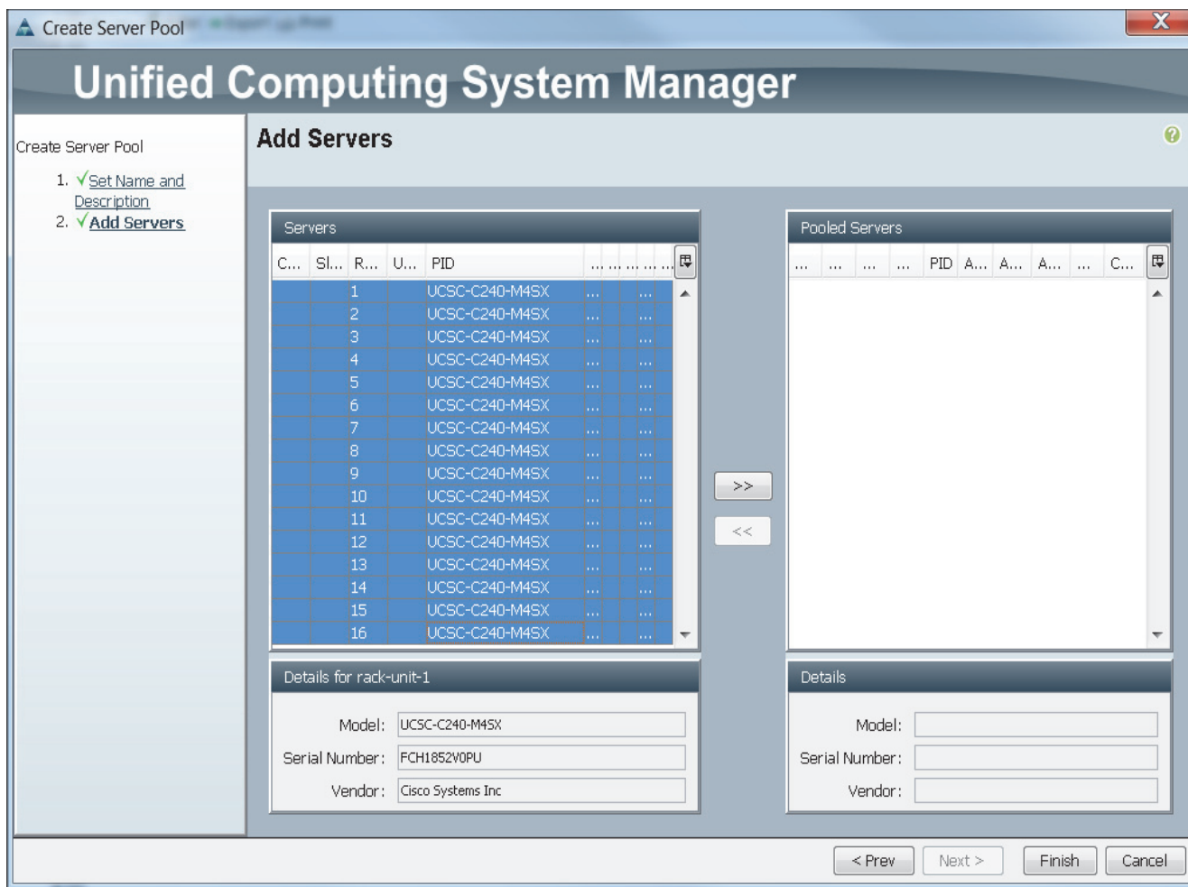
Figure 32 Adding Servers to the Server Pool
