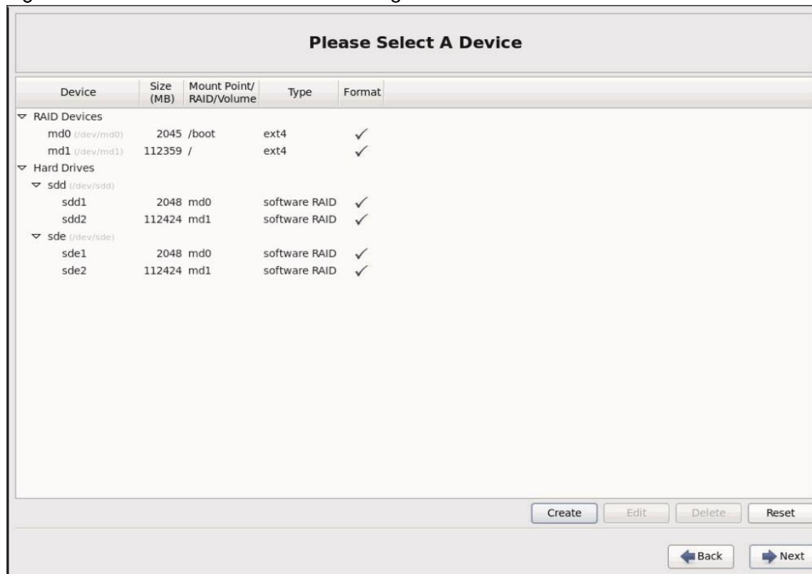
Figure 137 RHEL Installation: RAID Configuration- Device Selection
