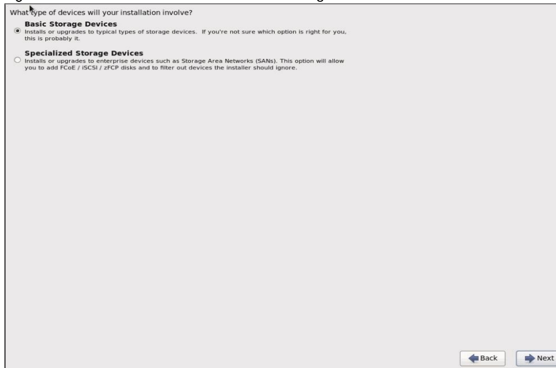
Figure 118 RHEL Installation: Select Basic Storage Devices
