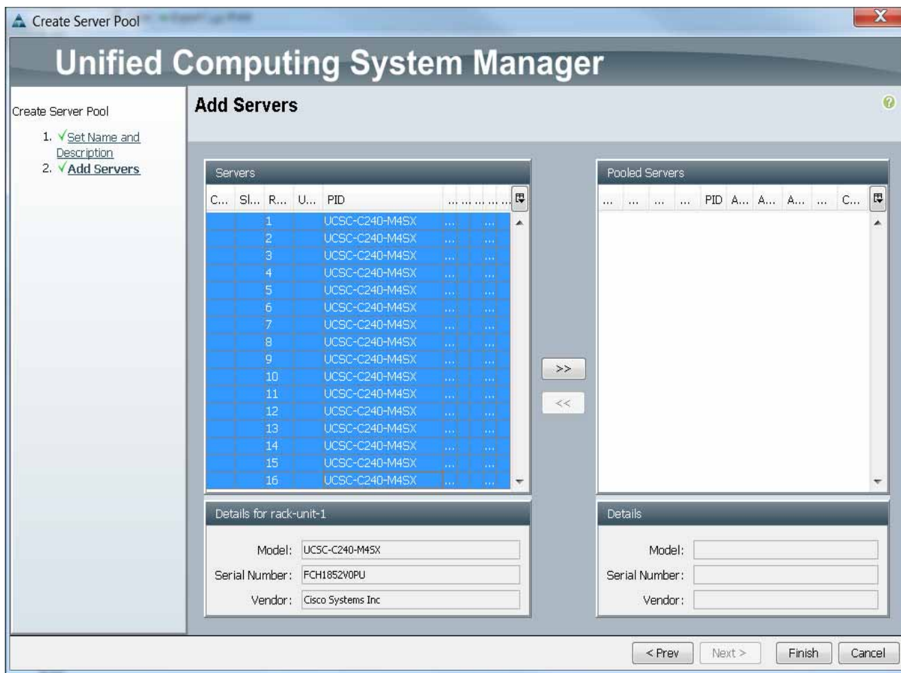
Figure 23 Adding Servers to the Server Pool
