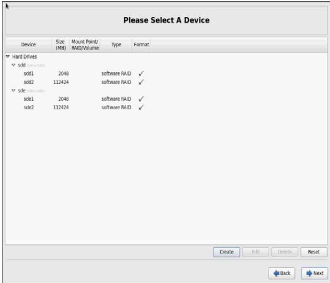
Figure 153 RHEL Installation: Selected RAID Devices
