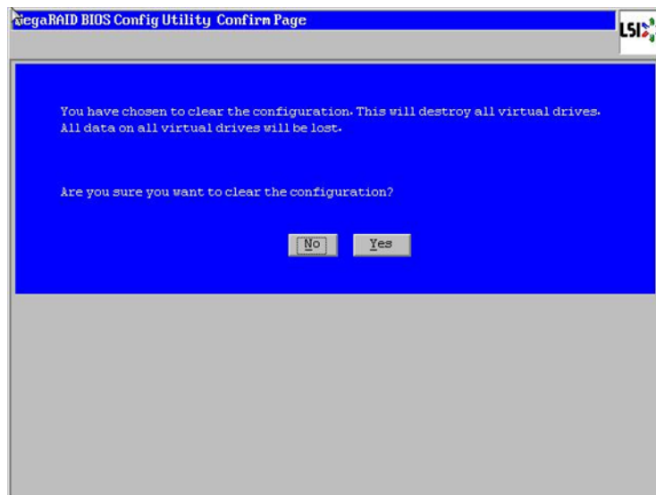
Figure 48 Confirming Clearance of the Previous Configuration on the Controller
