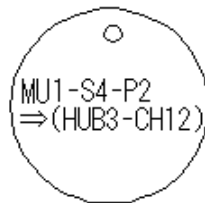
Figure I-3 Cable destination label with tie
