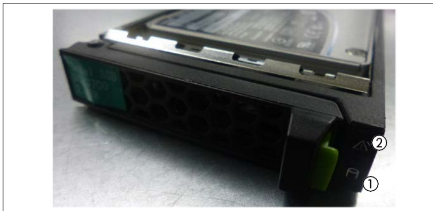
Figure 6.7 Indicators on a hot-plug PCIe SSD SFF module
