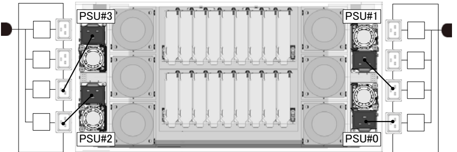
Figure 5.6 Connecting Diagram of PSU Redundant(2+2) with AC Redundant
