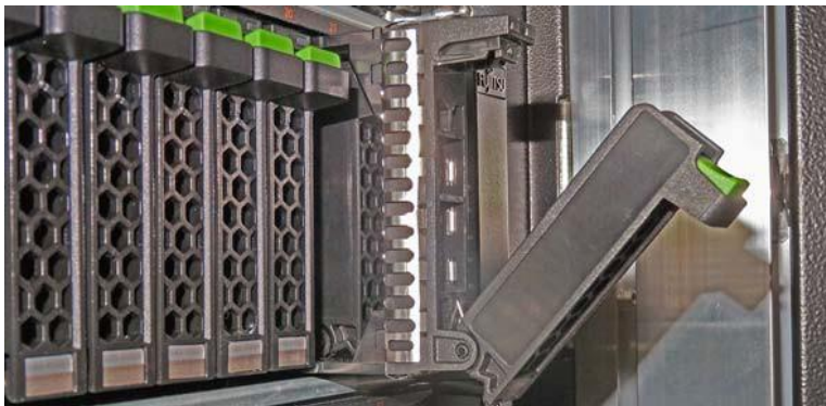
Figure 17: Removing/installing a 2.5" hard disk drive
