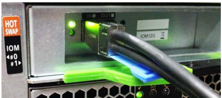
Figure 19: Orientation of the Mini SAS HD plugs
