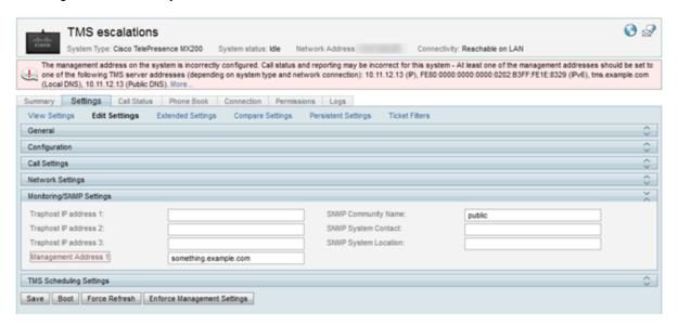
The Systems > Navigator window for a system with an incorrect management address.
