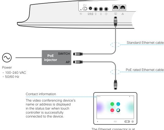
The Ethernet connector is at the rear of the touch controller.
