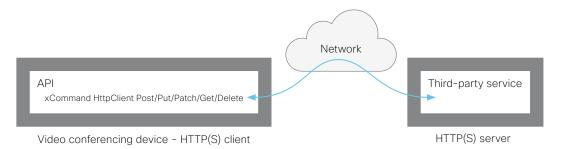
The HTTP(S) request feature makes it possible to send arbitrary HTTP(S) requests from a video conferencing device to an HTTP(S) server. Furthermore, the device receives the response that the server sends back. The device supports the Post, Put, Patch, Get, and Delete methods.
