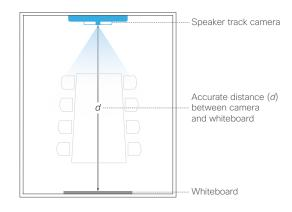
The whiteboard must be placed across the room from the camera, as shown in the illustration.
