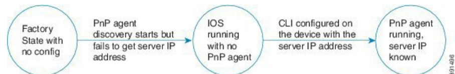
Figure 4: Workflow for PnP Trigger with CLI Configured PnP Profile
