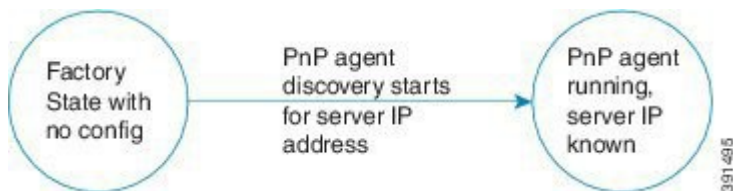
Figure 3: Workflow for PnP Trigger with no Startup Configuration
