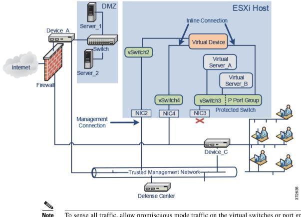
To sense all traffic, allow promiscuous mode traffic on the virtual switches or port groups where the device sensing interfaces connect. See Configuring Virtual Device Interfaces, page 3-9.
