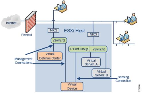
Your sensing connection on your virtual device must be allowed to monitor network traffic. The virtual switch, or the port group on that switch to which the virtual interface connects, must accept promiscuous mode traffic. This permits the virtual device to read packets intended for other machines or network devices. In the example, the P Port Group is set to accept promiscuous mode traffic. See Configuring Virtual Device Interfaces, page 3-9.
