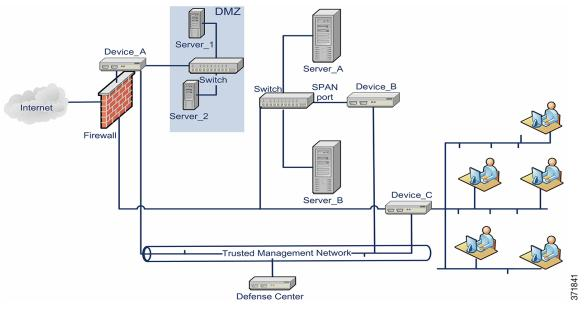
You can configure port mirroring on most network switches to send a copy of network packets seen on one switch port (or an entire VLAN) to a network monitoring connection. Also called Switch Port Analyzer or SPAN by a major network equipment provider, port mirroring allows you to monitor network traffic. Note that Device\_B monitors the traffic between Server\_A and Server\_B via a SPAN port on the switch between Server\_A and Server\_B.
