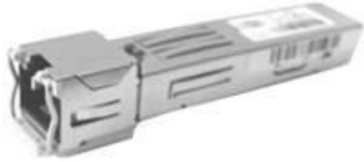
Figure 2 - Cisco 1000BASE-T Copper SFP (GLC-T)
