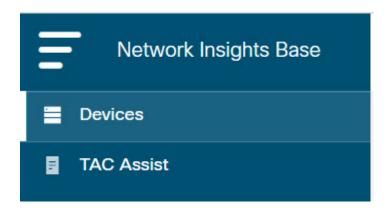
1 Devices: Sorts devices by device name, serial number, IP address, version, and platform.
