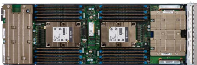
Figure 23. Cisco UCS B200 M5 Blade Server with two P6 GPU cards
