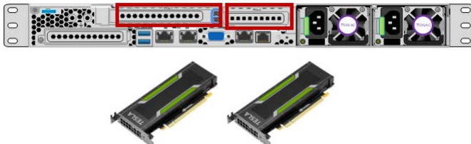
Figure 21. NVIDIA Tesla P4 installation on Cisco UCS C220 M5
