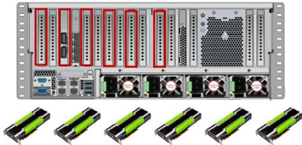
Figure 22. NVIDIA Tesla P40 installation on Cisco UCS C480 M5
