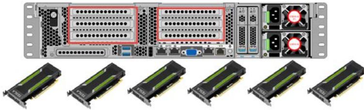
Figure 20. NVIDIA Tesla M10 or P40 installation on Cisco UCS C240 M5
