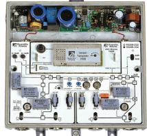
The pilot frequencies are selectable and may be altered on site according to the actual channel load – no factory set pilot frequencies!
