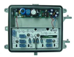
The amplifier performs to 1 GHz in the forward path and can be configured electronically by using a handheld programmer
