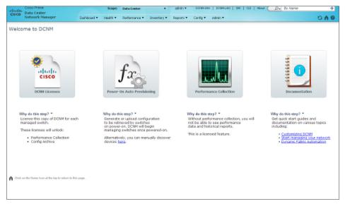
Figure 2. Cisco Prime DCNM Dashboard
