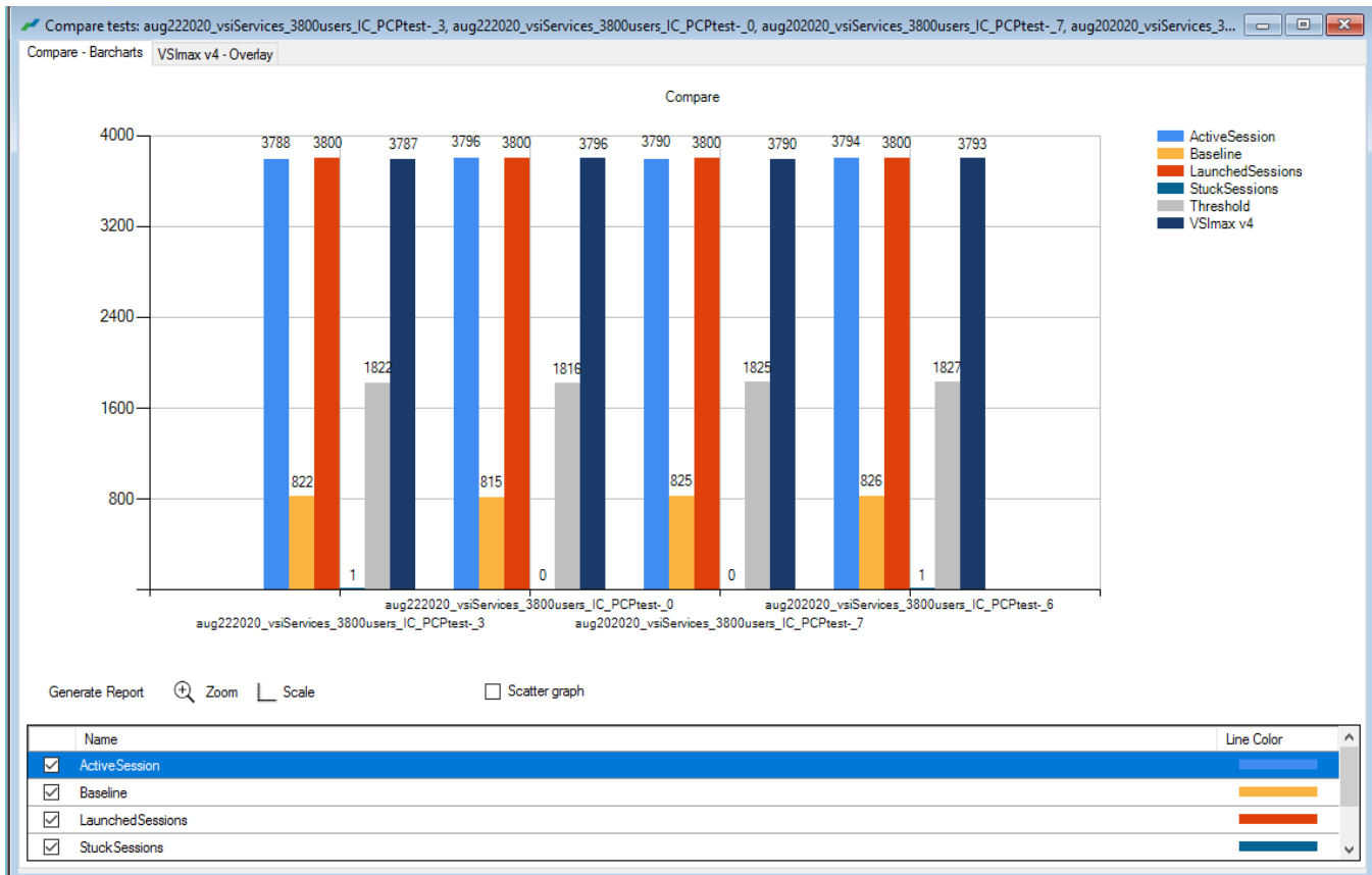
Figure 59 Three Consecutive Login VSI Analyzer Chart for 3800 Windows 10 VMware Instant Clone Non-Persistent Virtual Desktops
