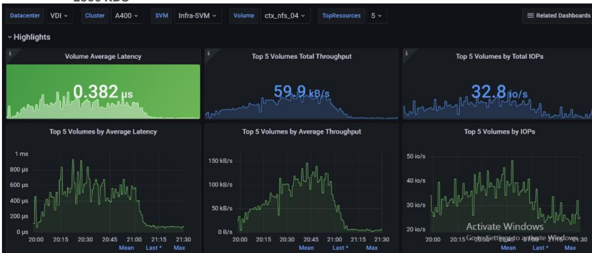
Figure 79. Volume Average Latency, Volume Total Throughput and Volume Total IOPS AFF A400 volume 4 for 2500 RDS
