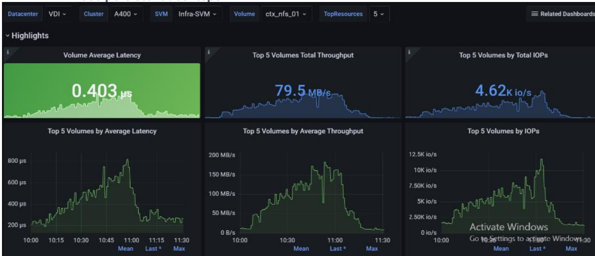
Figure 81. Volume Average Latency, Volume Total Throughput and Volume Total IOPS AFF A400 volume 2 for 2000 persistent desktops
