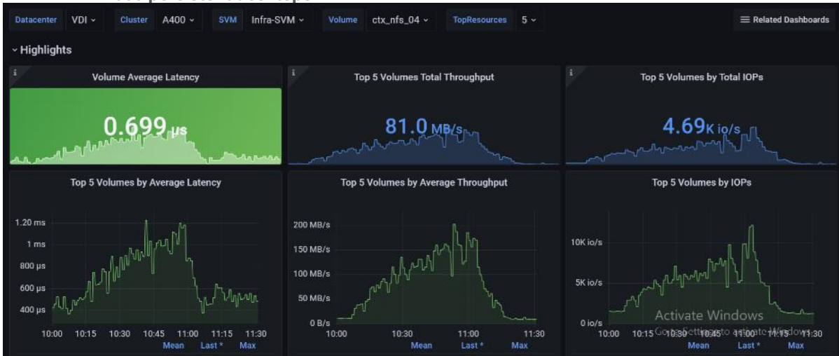
Figure 83. Volume Average Latency, Volume Total Throughput and Volume Total IOPS AFF A400 volume 4 for 2000 persistent desktops
