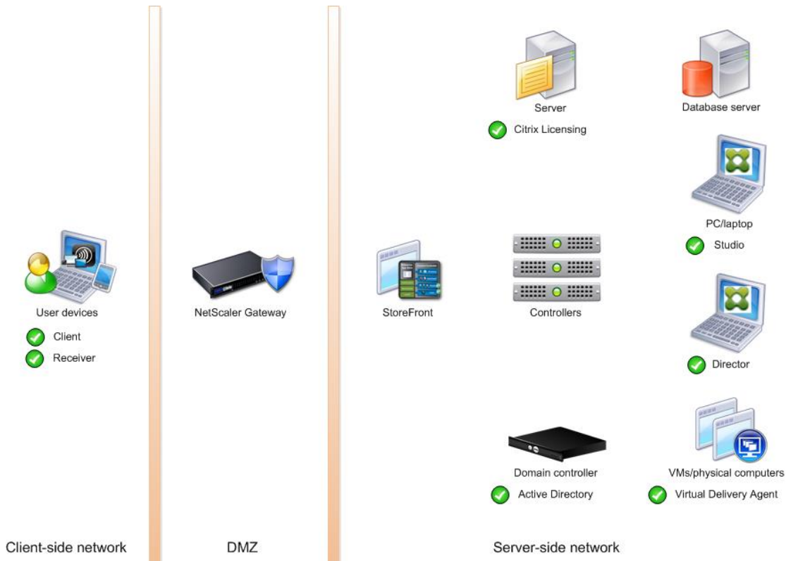
Figure 11. Example of a Distributed Components Configuration
