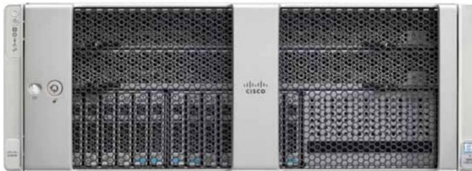
Figure 11 Cisco UCS C480 M5 Rack-Mount Server – Front View
