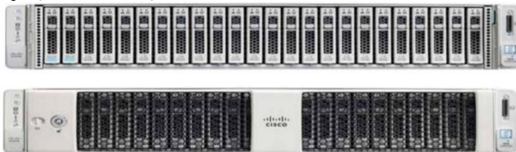
Figure 9 Cisco UCS C240 M5 Rack-Mount Server – Front View
