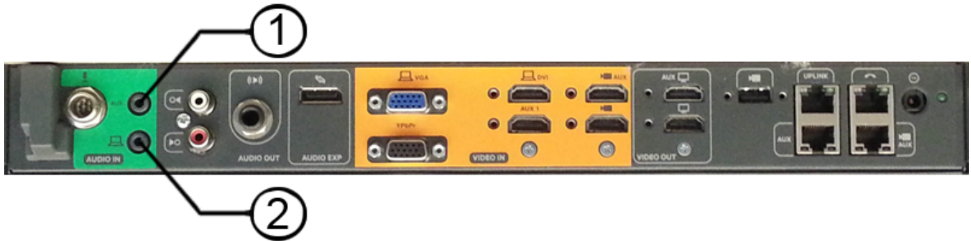
Figure 4-3 Audio Connections for the Presentation Cable
