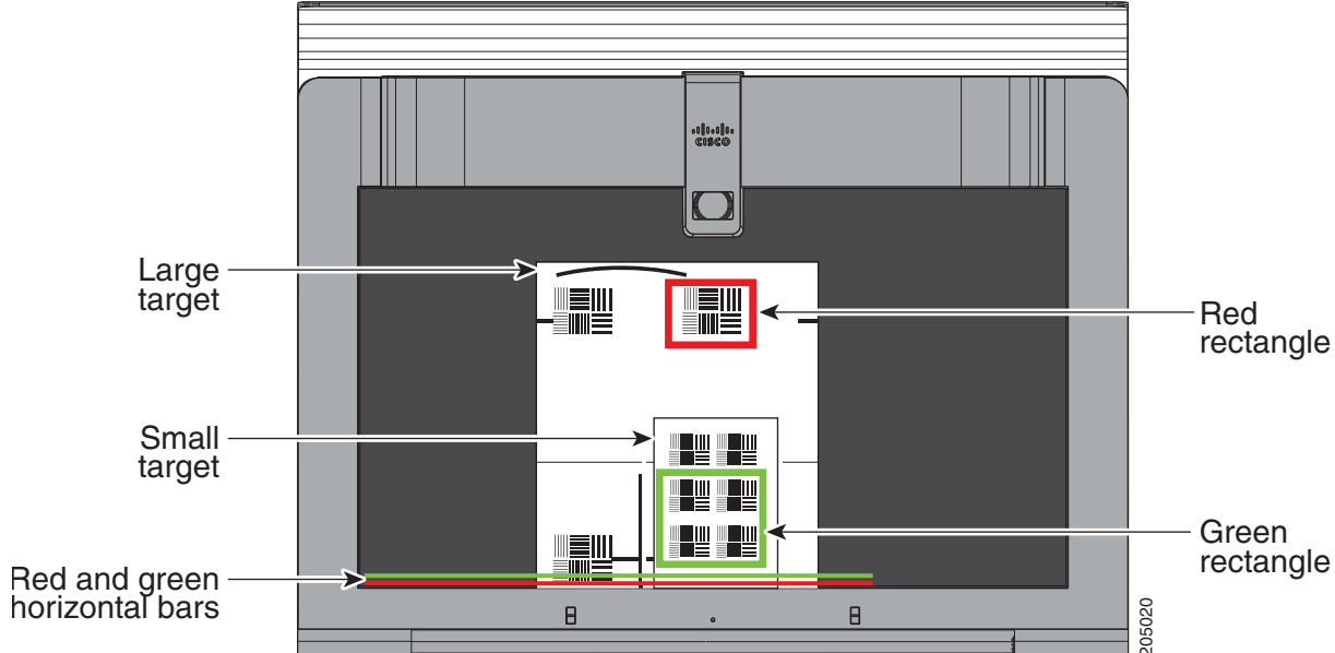
Figure 4-10 Setting Up Focus Targets and Aligning Horizontal Bars
