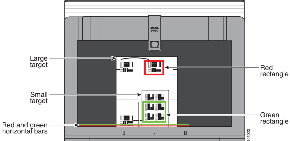
Figure 4-12 Setting Up Focus Targets and Aligning Horizontal Bars
