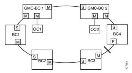
In a network with two GMC-BCs, the secondary GMC-BC can synchronize to both the NTP reference and the PTP reference at the same time, so the secondary GMC-BC can immediately take over when the primary GMC-BC fails. The GMC-BC instantly updates the time during a switchover.
