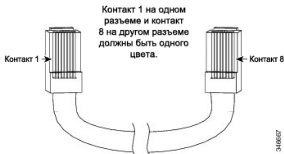
Figure 56: Identifying a Rollover Cable
