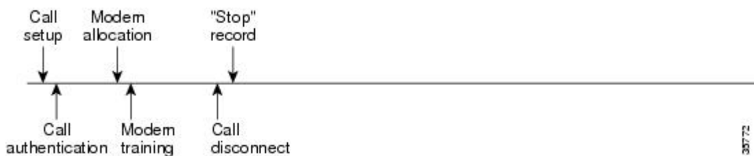
Figure 71: Modem Dial-In Call Setup Sequence With Call Disconnect Occurring Before User Authentication and With Resource Failure Stop Accounting Enabled
