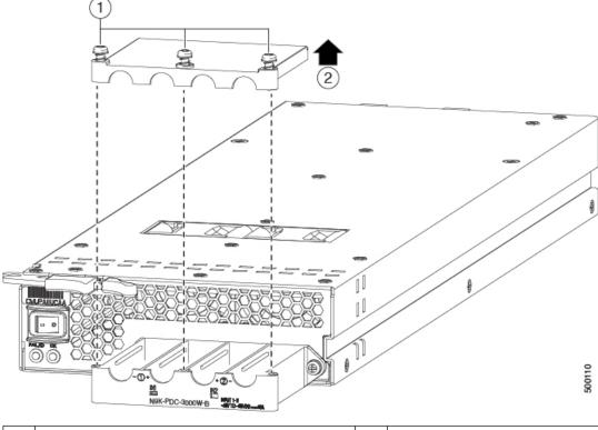
1 Remove 3 screws from the safety cover. 2 Remove the cover.
