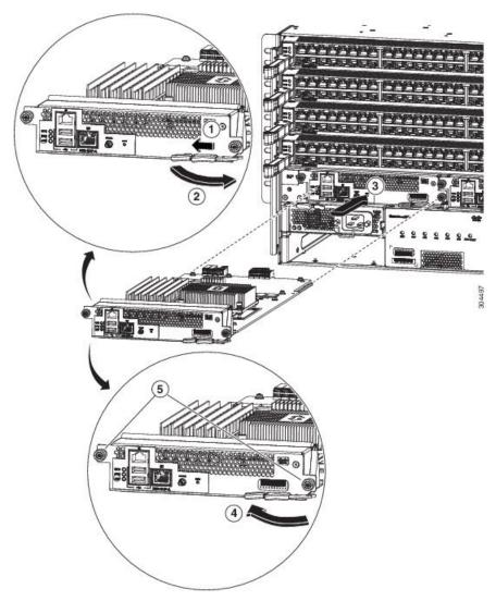
The module stops when its front is about 0.25 inches (0.6 cm) outside the front of the chassis.
