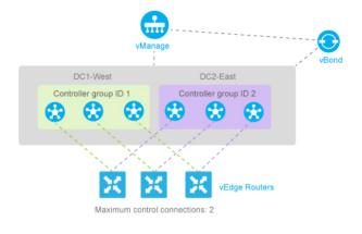
You configure the three vSmart controllers in DC1-West with controller group identifier 1:
