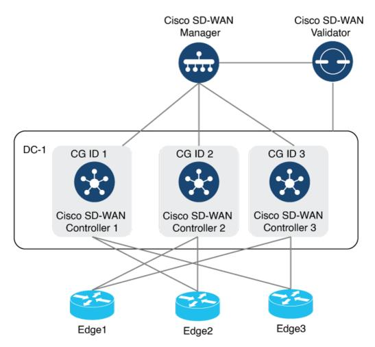
To display the control connections with the Cisco SD-WAN Controllers, use the **show control connections** command. The last column on the output, **Controller Group ID**, lists the Cisco SD-WAN Controller group that a router is in.
