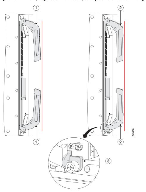
Figure 1-8 ISM (Integrated Service Module) Card Ejector Lever Positions During Installation
