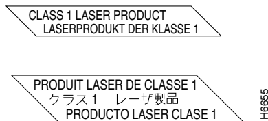
Figure 2-1 Class 1 Laser Warning Labels for Single-Mode Port
