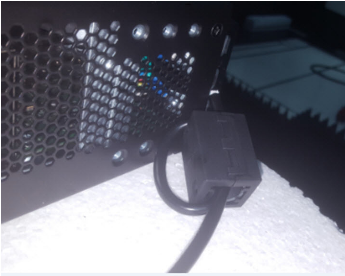
Figure 9 Secure Cable and Ferrite Clamp to Chassis
