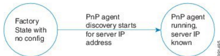
Figure 53: State Diagram for PnP Trigger with no Startup Configuration
