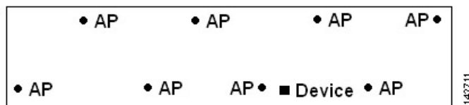
Figure 5: Improved Location Accuracy by Staggering Around Perimeter
