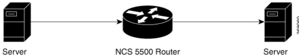
Figure 11: Topology for ERSPAN Egress Rate Limit
