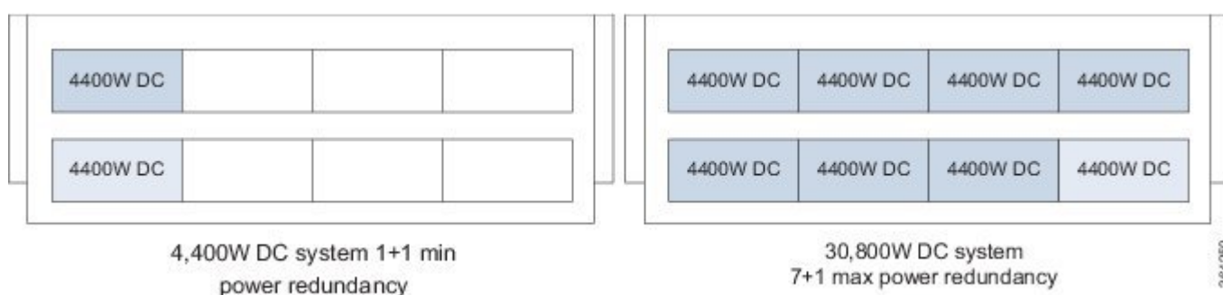
Figure 105: DC System Power Redundancy for the Cisco ASR 9010 Router—Version 3
