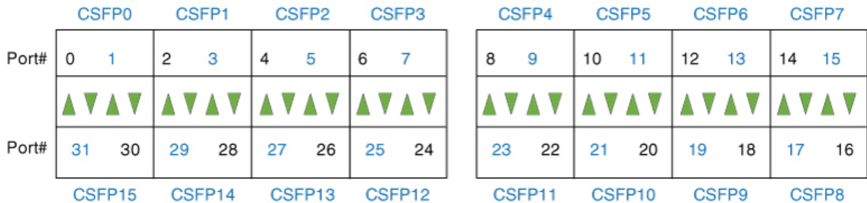
Figure 40: CSFP Ports on a 32-Port Gigabit Ethernet Modular Port Adapter with MACsec
