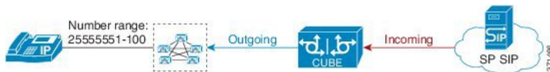
Figure 2: Incoming and Outgoing Messages Where SIP Profiles Can Be Applied
