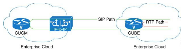
Figure 4: Anti-Tromboning - Avoiding Media Loops
